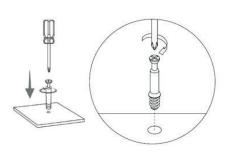
2. In the other panel, insert the cam lock and align it so it can properly receive the bolt, then join both panels (the cam locks might come pre-installed in this unit).
