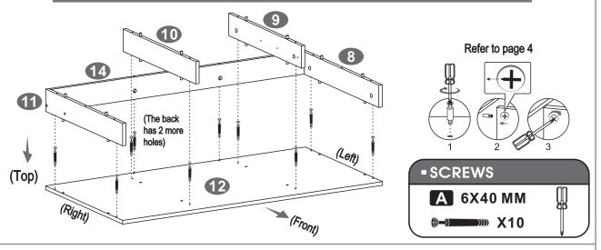
Open the sliders (9) slowly until you see the first hole on the back side of the slider thru the big opening, and using screws (11) assemble the sliders to the internal panels (9) and (10) on the front as shown.
