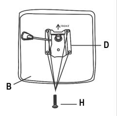
Place the top parts over the base parts making sure the tip of the gas lift enters into the hole of the mechanism.
