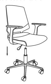
Use screws (I) and washers (J) to assemble the backrest (A) to the seat (B) as shown.
