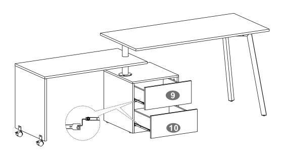
■Tighten any and all screws. Insert the drawers into the cabinet, starting with the bottom drawer. You might have to insert it at a downward tilted angle.
