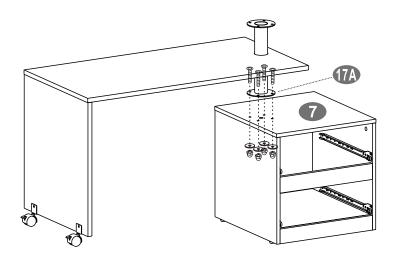
•Use screws I, J & K to assemble the Rotating Structure (17) to the Top Panel (7) as shown.
