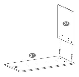
•First screw bolts B to the Small Table Top (24), then assemble it to the Big Side Panel (25) as shown and as explained in page 5.
