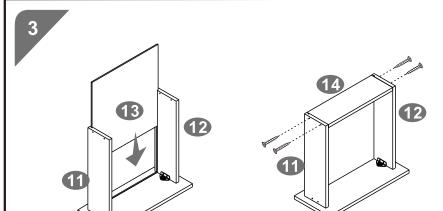
Slide in the Drawer Bottom Panel (13). Use screws E to assemble the Drawer Back Panels (14) to the Drawer Left and Right Panels (11 & 12).
