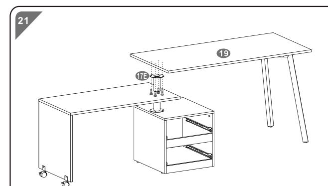
■Use screws D to assemble the Rotating Structure (17) to the Big Table Top (19).
