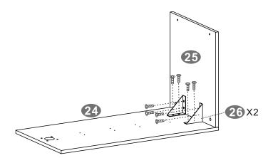
•Use screws D to assemble the Support Structures (26) to the Small Table Top and Big Side Panel (24 & 25).
