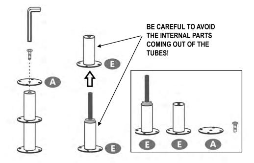
Assemble the bottom tube "E" to the auxiliary panel (24) using screws (D) as shown.
