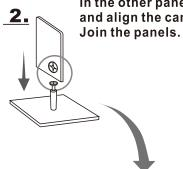
In the other panel, insert and align the cam lock.
