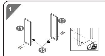
Use screws A to assemble the Drawer Connects (15) to the Drawer Left and Right Panels (11 & 12).
