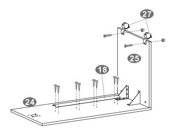
•Use screws C to assemble the Support Tube (18) to the Small Table Top (24). Use screws I & J to assemble the Casters (27) to the Big Side Panel (25).
