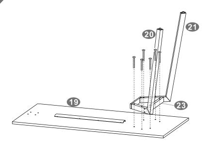
•Use screws H to assemble the Back Structure, Front Structure and Long Connect Tube (20,21 & 23) to the Big Table Top (19).
