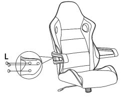
Place the top parts over the base parts making sure the tip of the gas lift enters into the hole of the mechanism.
