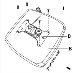
Using screws (J), assemble the backrest (A) to the seat (B) with its metal plate on top of the mechanism (D) as shown.
