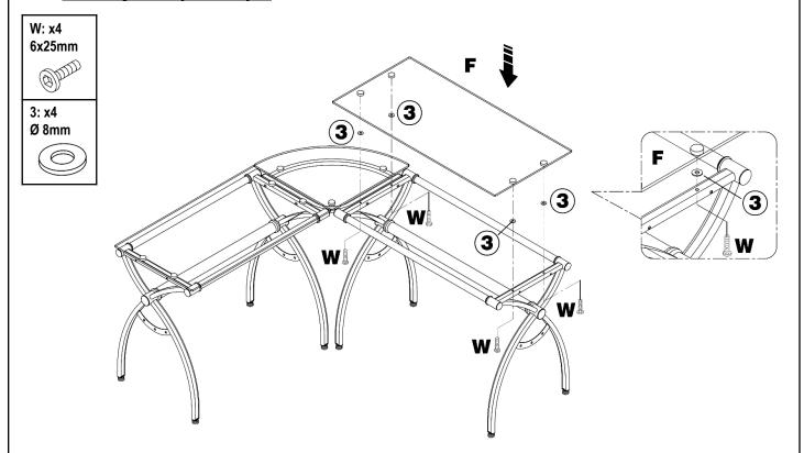
Please keep in mind that the glasses won't necessarily align perfectly, and might look a little uneven or small gaps might occur. This should not be considered a defect unless the gap or misalignment is by more than a quarter of an inch (8mm). You can try improving the leveling and close the gaps as much as possible by adjusting the unit manually as shown below. Once the adjustments have been done, **you can proceed to tighten all the screws.**
