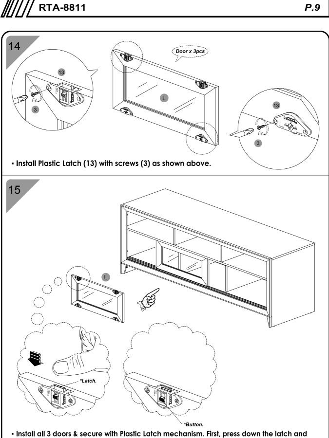
press down the button. Then place all doors into the cabinet, once secure in place push the button up to release the latching mechanism.
