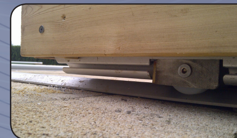
• Brake with rubber pad and guide wheel
