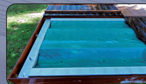
• Protective membrane to limit evaporation
