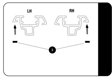
Fit the Foam Strips (Item 3) by removing the double-sided tape and applying them to the outside profile edge of each of the Tracks as shown in 2.3.
