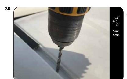
Before drilling the holes in the roof, you need to do a bit of prep. Take both the 3 mm and 5 mm drill bits. Using a suitable tape, wrap a band of tape around the drill bit to act as a stopper to prevent you from drilling to deep as there are airbags located below where you will be drilling.
