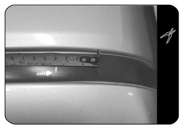
C) Looking at the rear of the ditch molding, measure 40mm from the joint line and make a mark
