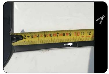
Looking at the front of the ditch molding, measure 100mm from the front and make a mark
