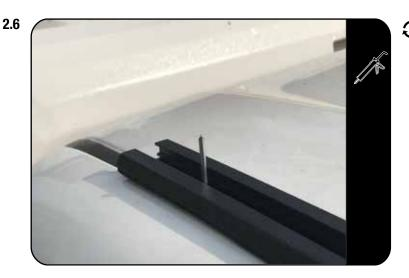
Place silicone sealant in and around each of the holes drilled.
