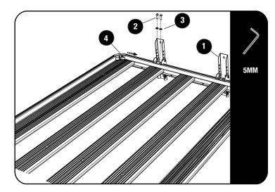
Slide 4 M8 nyloc nuts (item 4) into the side profile as shown and loosely fit the Rotopax side mounting brackets (item 1) with the fasteners shown.
