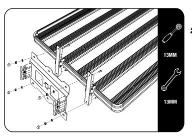
Fit the Rotopax mounting plate to the Rotopax side mounting brackets. Move the side mounting brackets to the desired position before fully tightening all the fasteners.
