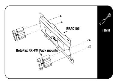
Fit 2 RotoPax RX-PM Pack mounts to the Rotopax mounting plate (RRAC105). Fasteners are supplied with the RotoPax RX-PM Pack mounts.
