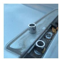
Clean out the areas around the mounting holes and make sure there is not debris in the area. You can also clean the area where the factory rack contacted the roof.
