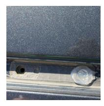
Add a glob of silicone or RTV sealant right over the top of the holes and then place the spacers into the silicone. The vehicle is now ready for you to install the rack.
