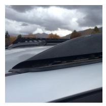
The covers are held by 3-4 clips along the edge so pry in multiple locations until the cover pops off.
