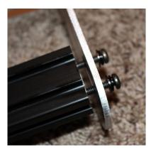
Start by connecting the crossbars to the side rails. Install the front, rear, and middle crossbars first to ensure that the rack is square. Tighten all crossbars loosely as shown in the picture and then go around and tighten them in even increments.
