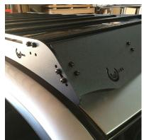
Once all tnuts have been fed into the channel and the extrusion bar and deflector are flush on both ends, turn the assembly over and tighten the screws till the lock washers are compressed. The defelctor can now be bolted to the rack.
