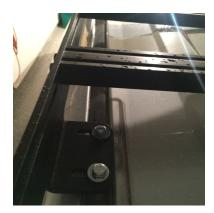
Secure the rack to the truck by using the 8M x 1.25 Hex bolts, lock washers and flat washers. Make sure to attach the rack loosely at all points before tightening any.
