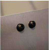
Complete step 3 for all ten mounting holes on the the wind deflector. The correct order is screw, lock washer, flat washer, deflector, tnut. The screw should be loosely threaded into the tnut.
