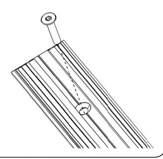
On the remaining ten threaded holes in the front and the rear of the roof, place some silicone on each hole. Insert a M6 x16 Button Head Bolt and M6 x19 x1 Flat Washer (Items 5& 6) into each hole and tighten using a 4 mm Hex key.
