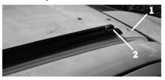
( C ) Using a marking pen, mark the two non threaded holes for both Tracks onto the vehicle's roof and remove the Tracks from the roof.
