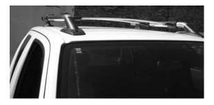
( **B** ) Place the Track (Item 2) on the roof, pick up the second threaded hole from the front and line up the two threaded holes at the back.
