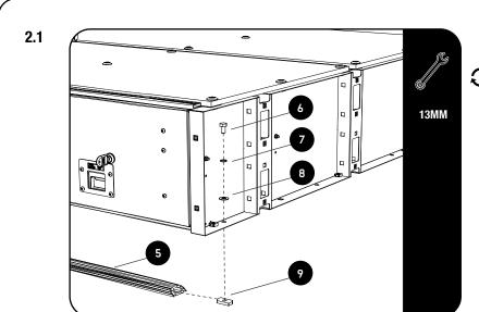
Slide 2 channel nuts (Item 9) into the track (Item 5). Center the track under the drawer and secure with the fasteners as shown.
