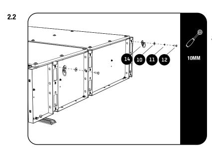
Secure the four D-Rings (Item14) on both sides of the drawer using the fasteners shown.
