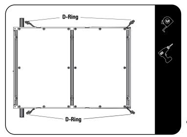
Place the drawer into the vehicle and center. Making sure the turnbuckles are pulling outward to prevent the drawer from moving after it has been secured.
