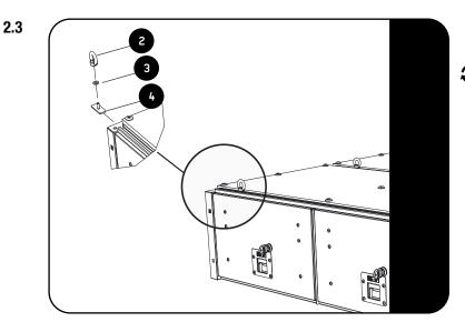
Assemble the eye-nuts (Item 2) with a M6 nylon washer (Item 3) and a stud plate (Item 4) and slide them into place.
