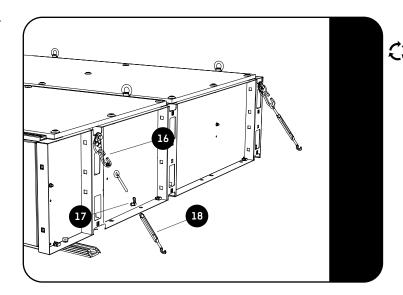
Assemble each of the 4 turnbuckles (Item 18) with a wing nut (Item 17) as shown. The wing nut will be used to lock the turnbuckles after they have been set.
