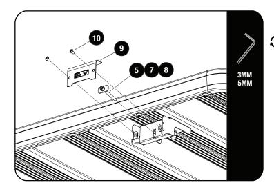
Remove the Front Covers (Item 9) from all the Grab-On Feet (Item 2) by loosening the two M5 x 10 Button Head Screw (Item 10).
