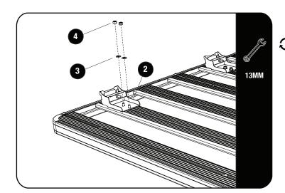
Fit the Grab-on Foot assembly (Item 2) to the slat by loosley fastening it with two M8 Flat Washers (Item 3) and two M8 Nyloc Nuts (Item 4).
