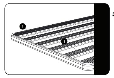
Place your Front Runner Roof Rack onto your vehicles Flush Rails and find the best position. The Rack should sit level to the ground, not the vehicles roof line.
