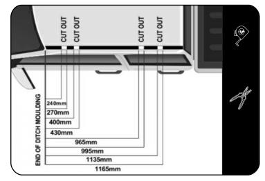
Starting at the front of the vehicle's roof, measure and mark the dimensions as shown onto each of the ditch mouldings.
