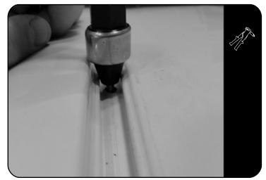
Using a Rivnut Tool, insert an M6 Rivnut (Item 10) into each of the eight 9mm holes drilled in Step 2.3.
