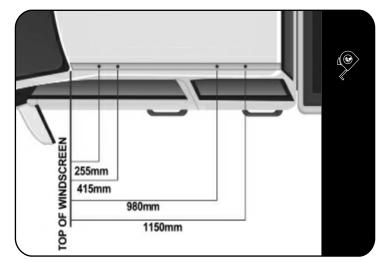
Make the following four markings as shown in the center of each ditch in the vehicle's roof.
