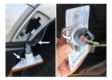
**STEP 5:** Removal of the turn signal is required for installation of front Fender Flares. Pull back the inner wheel well liner to locate the turn signal body and wiring. Remove the turn signal from the vehicle body by squeeze the lower tab on the back of the turn signal body. Carefully turn the wiring harness counter clockwise and remove the bulb-wiring harness from the turn signal body.
