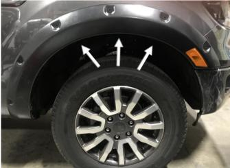
**STEP 8:** Reconnect the bulb-wiring harness to the turn signal body, place the Fender Flare onto the vehicle into position of best fit. To secure the Fender Flare to the vehicle body, install the provided screws and washers into the screw plugs in the three shown locations.
