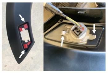
**STEP 6:** Apply the provided tape squares 3 per side to the turn signal recess, cutting of the tapes will be required per image. Remove the tape liner, install the turn signal body into the recess in the front Fender Flares. Ensure the tabs in the back of the turn signal body snap into the Fender Flare recess pocket. Apply firm pressure across the trun signal once in place to achieve tape wet out. Reinstall the bulb-wiring harness to the turn signal body.
