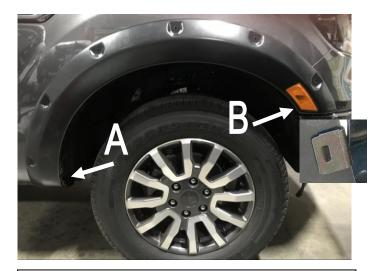
**STEP 9:** Apply upward tension on Fender Flare to the vehicle fender when installing the large U clip in location A and the small U clips in location B. Slide the clips over the Fender Flare and the inner wheel arch lip in the two locations shown. Position the clip so that the barb in the clip locates in the slot of the Fender Flare. Ensure all fixing points are tight and secure and that the rubber seal is flush neatly against the vehicle body. Repeat install steps for the opposite side.
