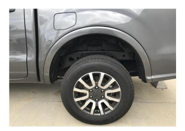
**STEP 12:** Clean the body areas where the Fender Flares will make contact. Ensure fenders are dry prior to install.
