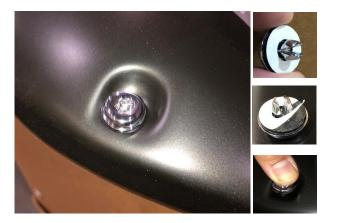
**STEP 1:** Attach the extruded plastic bolts. Peel back white tape liner from the bottom side of the extruded plastic bolt and press until it snaps into place. Ensure inside of Fender Flares where the rubber seal is attached is clean, using the alcohol wipes provided. Wipe away any residue with a dry clean cloth.
