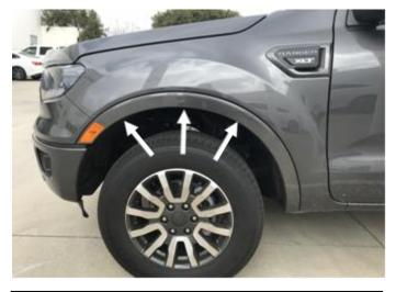
**STEP 7:** Using phillips head screwdriver remove factory wheel arch fasteners in the three shown locations. Install the screw plugs provided in the hardware kit into the shown locations.
