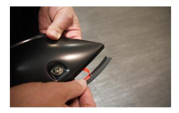
**STEP 11:** Attach the included rubber seal to the Fender Flares. Peel Back 2" of the adhesive backing and position on the Fender Flare. Attach the seal to the Fender Flare, peeling back a few inches at a time. Ensure pressure is used to secure rubber seal to the Fender Flare edge. Attach rubber seal along all areas the Fender Flare will make contact with the vehicle body. Trim excess rubber seal.
