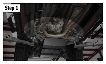
If you have the Cali Raised transmission skid, you will need to remove the (2) ½" carriage bolts that hold the rear position of the transmission skid.
