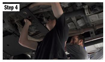
With a floor jack or a friend, lift the transfer case cross bar up and into position. You will need to lift the brake line bracket away from the frame to the cross bar can slide into place. Line up the holes on the driver side and put the bolt back in with a 12mm. Leave loose.
