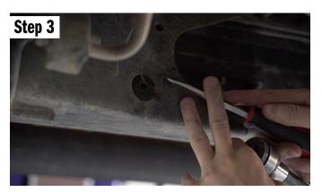
On the passenger side, in the same location there are (2) round black stickers on the frame. Using a screwdriver, remove the (2) black stickers revealing the (2) holes behind them.
