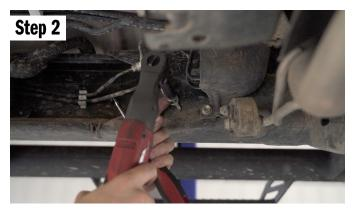
Next, we need to prep the frame for the transfer skid cross bar. On the driver's side of the frame, there is a bracket that holds on your brake lines. Remove the bolt that holds this bracket with a 12mm socket.
