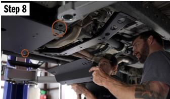
Now we can slide the transfer case skid in place. You will want to grab at least one  $\frac{1}{2}$ " carriage bolt, flat washer and lock nut. Slide the short end of the transfer case skid between the transmission skid and factory crossmember. Then pivot it up to your new transfer case cross bar. Taking the  $\frac{1}{2}$ " carriage bolt, put it through the skid plate and through the cross bar. Then put on a flat washer and lock nut.
