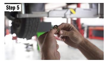
On the passenger side, line the cross bar up with the holes in the frame. Then grab a 3/8's bolt and put on a flat washer. Take the bolt and reach into the frame and push the bolt through the larger hole in the frame, then the cross bar. With the bolt in place, put on the 3/8's flat washer and lock nut.
