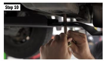
Moving to the front of the skid, take the longer ½" carriage bolts and push then through the transmission skid (if installed), then the transfer skid, then the crossmember and finally through the backing plate. Install a ½" flat washer land lock nut. Do this for both sides.
