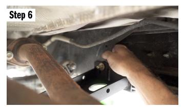
With the cross bar in place, apply pressure upward ensuring it contacts the frame. Then tighten the drivers side bolt with your 12mm. Then move to the passenger side and tighten that hardware with a 9/16 socket and wrench.
