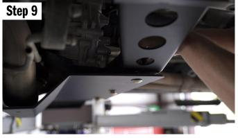
Put in the remaining (2) carriage bolts with a flat washer and lock nut. Leave these all loose.
