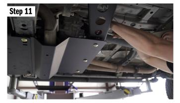
With all of the hardware installed, adjust and align your skid plate with all of your other components, then tighten all the nuts for the (5) carriage bolts. This completes your installation
