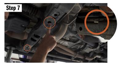
If you already have the Cali Raised transmission skid, you can skip this step. If you do not, place the rectangular backing plate on top of the factory cross bar over the (2) holes shown.
