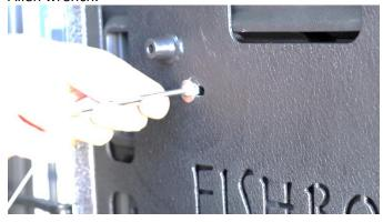
Finally, with the larger bolt and washer, secure the bottom drilled hole with a 5mm Allen Wrench.
