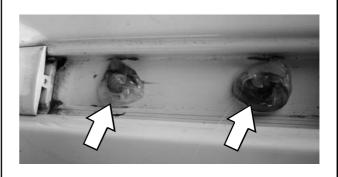
Place a Spacer (Items 8) into each of the Mounting Point Recess, lining up the holes in the Spacers with the bolt holes in the roof. Ensure that the wide section of the Spacers (as indicated in the image) go towards the outside of the vehicle.
