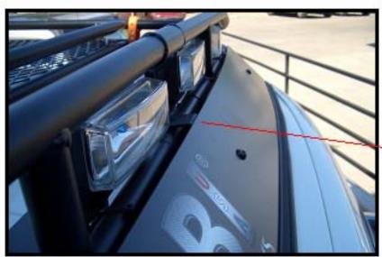
Prior to install make certain all farring brackets are positioned so that the bend of the brackets are set equal to the top of the farring as shown to the left
