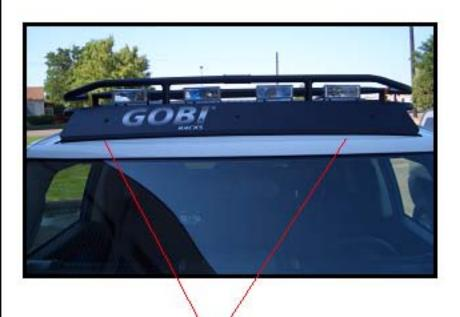
must be in contact with the vehicle roof top. If necessary you can bend a farring bracket or pull down on the rubber molding to achieve the final result.
