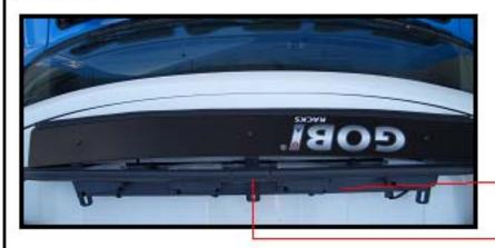
Place your farring onto the vehicle roof top then centered onto the Gobi roof rack light bar as shown to the left
