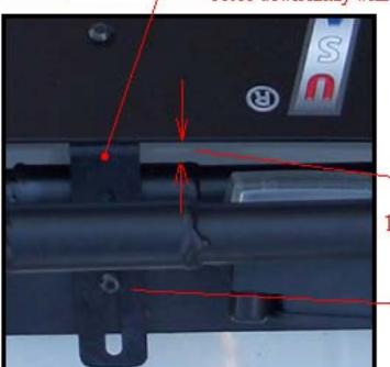
Provide approximately 1 to 2 inches of space between the lower front roof rack tubing and the farring and tighten down the farring bracket bolt. Press down firmly on the center bracket while tightening the bolt as this will provide a good tight seal between the farring and roof top
