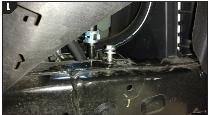
• Mount the re-location brackets as shown in photos (5/8” bolts under the A/C condenser factory bolts in factory location) – Photos M & N
