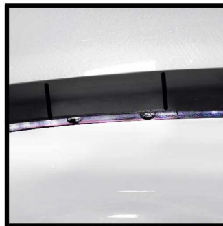
Next lay the trim parallel to where it was removed from and mark the area around the mounting holes to be removed
