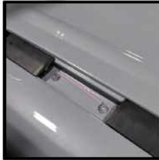
Next add the trim back to the roof around the mounting holes
