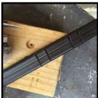
For the alternate trimming technique use an angle grinder or rotary tool to cut through the ...
