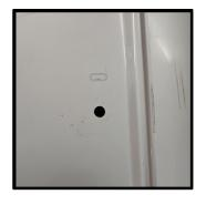
Work you way up to a 3/8" bit and then try to insert the plusnut. The recommended hole size from plusnut is .386"-.391"
