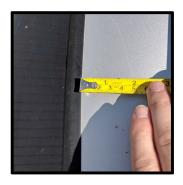
Measure back from the seam of the windshield as shown to a distance of 9<sup>1/4</sup>" and mark on the driver and passenger side
