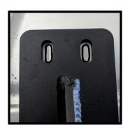
Install the front plusnut on each side of the vehicle and lightly bolt in the roof rack. Visualy inspect the fit. once satisfied mark the remaing slots to be drilled
