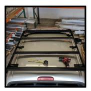
Fasten the remaing bolts and then attatch the last crossbars over the mounting feet
