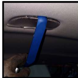
Remove cover from the next dome light.
