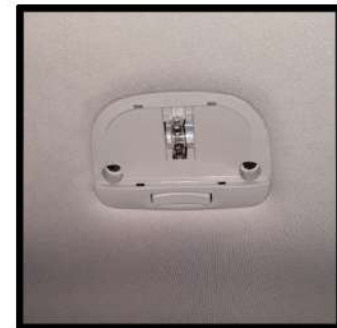
Remove the two philips head screws.
