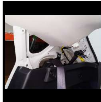
Rear paneling removed.
