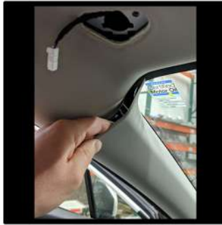
Pull back the top of the A-pillar trim.
