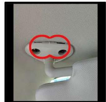
Next remove the two philips head screws circled above and use a flat head screw driver or trim removal tool to pop the visor out by prying up on the two small slots seen above.
