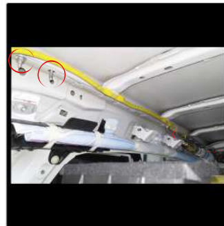
The bolts holding the roof rails in are now exposed and the nuts can now be removed.
