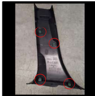
Now remove the lower B-pillar trim. Clip locations circled above.
