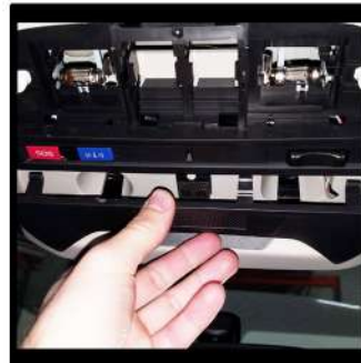
Begin removing the dome lighting from front to back.
