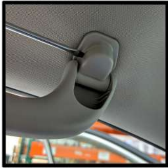
Begin removing the over head handles.
