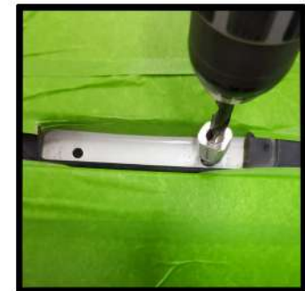
Now with the stock rails removed drill out the holes to 3/8". * Using a drill stop is recommended.
