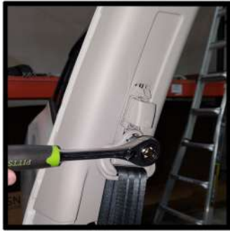
Remove seat belt. * When reattached the recommended tightening torque is 22.1 ft-lb
