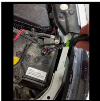
Before beginning the headliner removal first disconnect the battery
