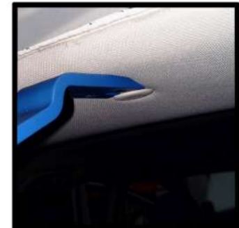
Lastly in the far rear there are three clips holding the headliner up.
