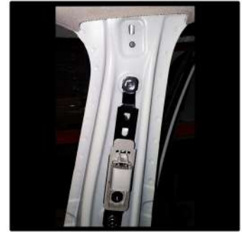
Upper B-pillar trim removed.
