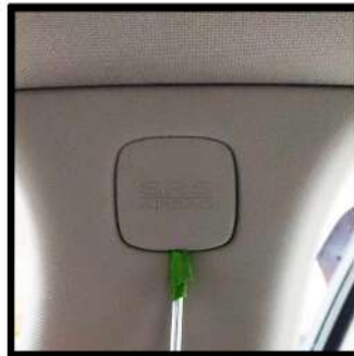
Now begin removing the B-pillar trim.
