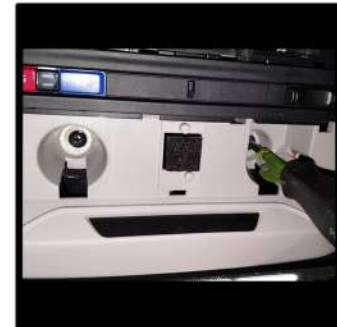
Remove the two philips head screws.
