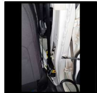
Lower B-pillar trim removed.
