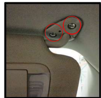
Remove the screws and drop down the visor. Undo any electrical plugs if necessary.
