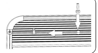
( **B** ) With your rack still upside down from Step 3A, slide a M8 x 20 Hex Bolt (Item 13) into the end of Slats 2, 5, 6, 10, 11.
