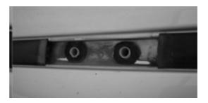
( **D** ) Clean the area around the threaded holes in the vehicle's roof using a rag and some methylated spirits / denatured alcohol. Place some silicone around each threaded hole in the vehicle's roof and the two cut-outs in each of the Spacers (Item 11) as shown. Position the Spacers into the vehicle's gutters, lining up the cut-outs in the Spacers with the threaded holes in the vehicle roof.
