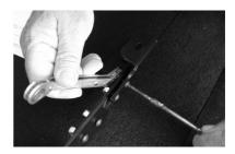
(B) Locate and remove the eight Plastic Covers (four each side) in the Ditch Moulding of the vehicle's roof. This is done my pushing the covers in the direction of the arrows found on the covers, and lifting.
