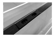
Place the Foot Rails onto the vehicle's roof, lining up the mounting holes in the bottom of the Foot Rails with the mounting points on the vehicle. The Product Sticker must go to the rear of the vehicle and must be facing outwards. Push the Foot Rails as far back as possible.
