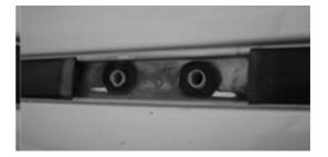
(C) Clean the area around the threaded holes in the vehicle's roof using a rag and some methylated spirits / denatured alcohol. Place some silicone around each threaded hole in the vehicle's roof and the two cut-outs in each of the Spacers (Item 8) as shown. Position the Spacers into the vehicle's gutters, lining up the cut-outs in the Spacers with the threaded holes in the vehicle roof.
