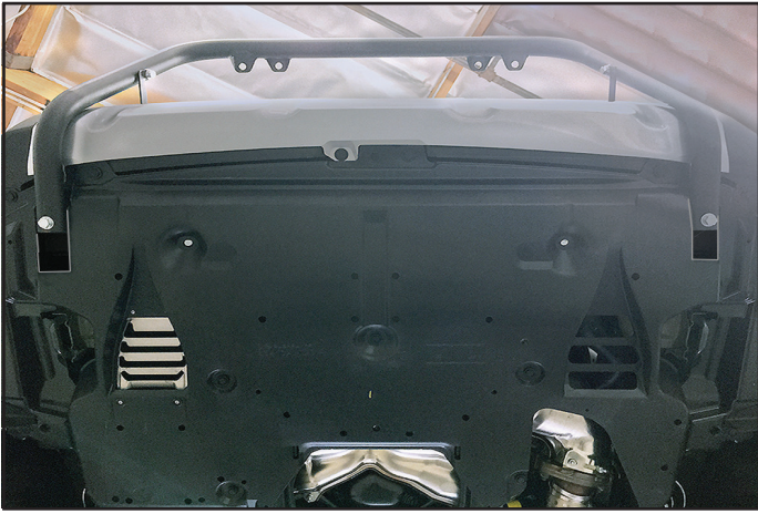
Reinstall engine splash shield.
