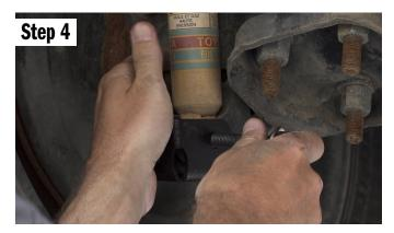
Take the shock skid and put the hex standoff in the 34" hole behind the shock. Then rotate the shock skid up and in position.
