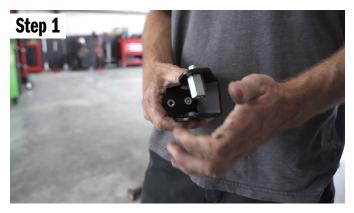
Get your ¼ bolt, split lock washer and flat washer. Put the lock washer on the bolt, then the flat washer. Then put the bolt through the mount. Then thread on the hex stand off. Tighten all the way with your allen tool and wrench.
