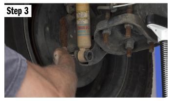
Remove the factory shock bolt. You can use a screw driver or pry bar to help keep the shock in position. You shock will try to extend making this a little difficult.
