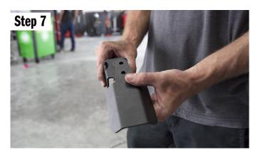
If installing the optional shock guard. Take two 1/4" inch bolts and install a lock washer and flat washer. Then line the shock guard holes up. Install the bolts and tighten.
