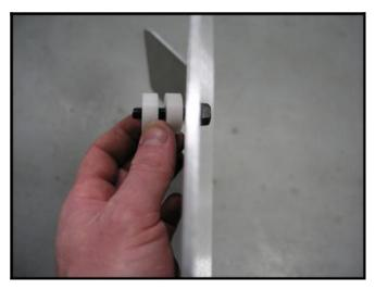
Position the skid plate up to the body of the vehicle and by hand, thread the new bolts in to the factory threaded holes that held the factory skid plate in position.
