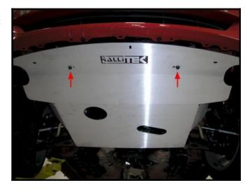
Install the rear hardware as shown on both sides. The rear hardware consists of four 10mm bolts, 4 washers, and four 10mm spacers.
