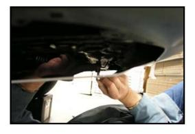
Attach the rear of the skid plate. For non-turbo applications use 40mm spacers and a 60mm long m8 bolt with washer. Skid plate ends will press tightly against sub frame when tightened. For turbo applications use 30mm spacers and a 50mm long m8 bolt with washer. Skid plate ends will press tightly against sub frame when tightened.
