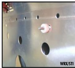
For turbo applications use the 20mm delrin spacers in the front of the skid plate. Place the spacer on top of one of the slots with a 40mm long m8 bolt with washer. Lift the skid plate into place and start the bolt by hand. Repeat on other front fasteners.
