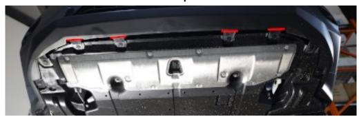
Tuck skid plate inside front bumper and install
