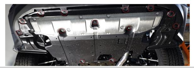
Cut factory tabs on front bumper on red lines. The RalliTEK skid plate tucks in the OEM bumper
