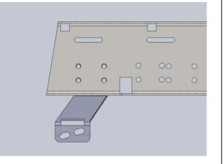
6. Take the rock slider base and brackets to their respective sides and start the bolts for the braces. The front brace will use the included M6x40mm bolts and the rear will use the included M10x30mm (no subframe drop) bolts or M10x70mm (with subframe drop) bolts. Install any subframe spacers between the rear rock slider brace and the subframe brace
