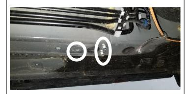
5. (OPTIONAL) NOTE: For a faster install you may let the bottom slider hang from the mounting bracket, attach the slider top to the base using supplied M6 button head bolts and serrated nuts (only a couple of threads on these bolts), support the slider to pinch weld, then use the slider as a template to drill the ½" holes in pinch weld (a right angle drill is recommended). Then skip to step 8.
