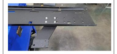
4. Take the rock slider base and brackets to their respective sides and start the bolts for the braces. The front brace will use the included M6x40mm bolts and M6 fender washers and the rear will use the included M8x30mm bolts and M8 washers.
