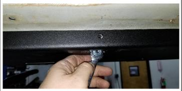
Once the bolts through the pinch weld are tight, tighten the bolts that go into the chassis, the 4 bracket bolts under the rock slider and the outer M6 screws. The nuts are serrated so you do not need to hold them while you tighten the bolts.
