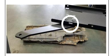
3. Install the braces onto the rock slider bases using the supplied M8 button head bolts, M8 fender washers, and serrated nuts as shown. Use washers between the button head bolt and mounting bracket, not between the serrated nut and slider. Be sure that the front brackets angle upwards from the base.
