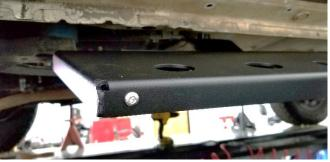
9. Rotate the rock slider assembly up in to place and use jack stands to support the rock sliders while you install the M6x40mm bolts through the pinch weld. Use a 10mm wrench to hold the nut through the cut out while you start the bolt from the inside of the pinch weld. Once all the bolts on one side are installed, tighten the bolts that go through the pinch weld.
