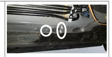
6. Rotate the rock slider base into position and mark the holes to be drilled in the pinch weld using a scribe or pick tool. It is helpful to support the front and rear of the rock slider base with jack stands while you mark the holes. Once you have marked the holes, remove the rock slider base and center punch near the bottom of the mark. Repeat the process for the other side.
