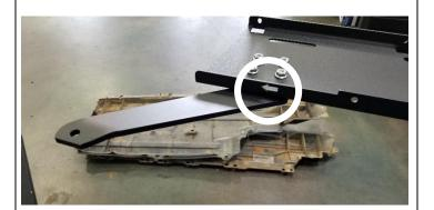
4. Install the braces onto the rock slider bases using the supplied M8 button head bolts and serrated nuts as shown. Be sure that the front brackets angle upwards from the base.
