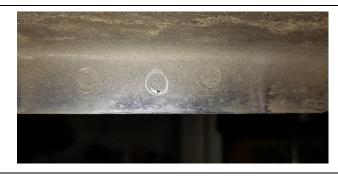
7. I recommend using a 1/8" drill bit to start drilling the mounting holes in the pinch weld and then stepping up to a 1/4" or 9/32" drill bit. Repeat the process for the other side.
