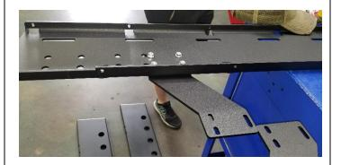
Take the rock slider base and brackets to their respective sides and start the bolts for the braces. The front brace will use the included M6x40mm bolts and the rear will use the bolts.
