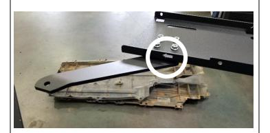
4. Install the braces onto the rock slider bases using the supplied M8 button head bolts and serrated nuts as shown. Be sure that the front brackets angle upwards from the base.
