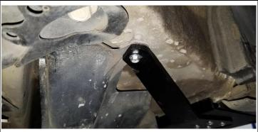
7. Rotate the rock slider base into position and mark the holes to be drilled in the pinch weld using a scribe or pick tool. It is helpful to support the front and rear of the rock slider base with jack stands while you mark the holes. Once you have marked the holes, remove the rock slider base and center punch near the bottom of the mark. Repeat the process for the other side.
