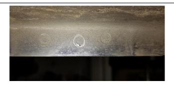
8. I recommend using a 1/8" drill bit to start drilling the mounting holes in the pinch weld and then stepping up to a 1/4" or 9/32" drill bit. Repeat the process for the other side.
