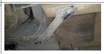
2010-2014 Models will need to remove the factory cover to reveal the front mounting point. You can find the covers on the frame supports at the back of the front inner fenders
