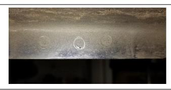
8. I recommend using a 1/8" drill bit to start drilling the mounting holes in the pinch weld and then stepping up to a 1/4" or 9/32" drill bit. Repeat the process for the other side.
