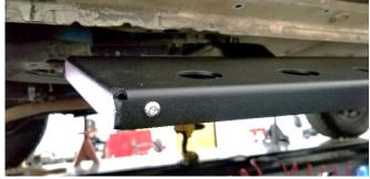
10. Rotate the rock slider assembly up in to place and use jack stands to support the rock sliders while you install the M6x40mm bolts through the pinch weld. Use a 10mm wrench to hold the nut through the cut out while you start the bolt from the inside of the pinch weld. Once all the bolts on one side are installed, tighten the bolts that go through the pinch weld.
