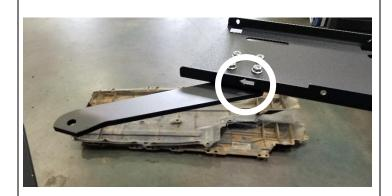
5. Install the braces onto the rock slider bases using the supplied M8 button head bolts and serrated nuts as shown. Be sure that the front brackets angle upwards from the
