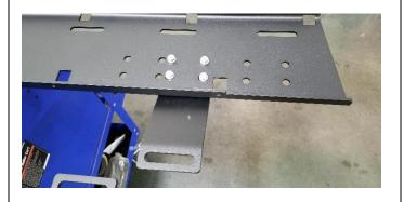
6. Take the rock slider base and brackets to their respective sides and start the bolts for the braces. The front brace will use the included M6x40mm bolts and the rear will use the included M8x40mm bolts. Install the included spacers between the rear rock slider brace and the chassis brace
