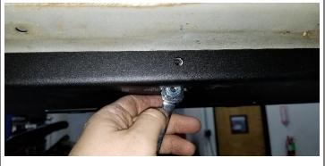
NOTE: the rock sliders may need to be manipulated up or down to get the bolts to start into the nuts. I recommend applying a little tape to keep the nut on the wrench during this process.
