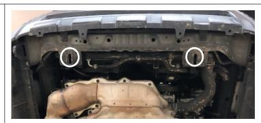
3. Insert the u-nuts onto the mounting plates and slide them into the factory bracket as shown.
