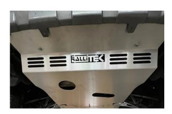
7. Slide the supplied 20mm spacers between the skid plate and sway bar support bracket one at a time and begin installing the M10x1.25x35 bolts
