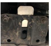
4. Remove the two bolts securing the sway bar support bracket to the subframe
