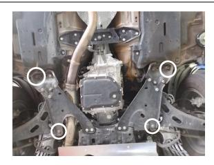
Hold the skid plate up and start the smaller 50mm long bolts in the front holes. Once those are started, start the larger 70mm long bolts in the rear holes. Once all 4 bolts are started, you can tighten them.
