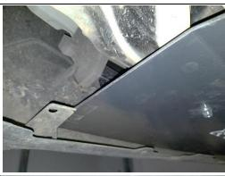
4. Move to the rear of the skid plate and install the 50mm long bolts to the threaded hole in the rear of the subframe. NOTE: Tighten the front bolts first and the rear bolts second.
