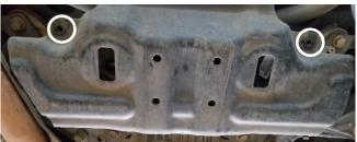
3. Slide the skid plate on top of the bottom of the bumper and start the 30mm bolts in the front holes
