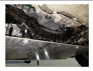
5. Optional – Install 2 of the clips that held the factory splash guard into the remaining holes in the skid plate
