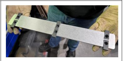
7. Place the oil filter panel mounts on top of the opening on the skid plate, then thread in the button head fasteners to secure
