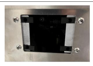
10. Install the oil filter and oil drain panels as shown using the supplied button head fasteners
