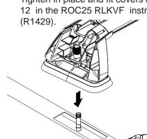
Locate M6 screw into stud. Tighten plastic bolt housing alternately both sides. Tighten 3-4 Nm.
