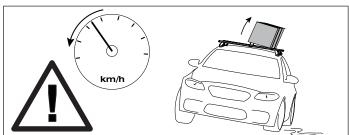
The handling characteristics of the vehicle changes when you transport a load on the roof. For safety reasons we recommend you exercise extreme care when transporting wind-resistant loads. Special consideration must be taken into account when cornering and braking.
