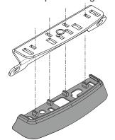
Locking points push through and fix onto Bracket.
