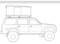
When these roof racks are to be used on a vehicle that is driven off sealed roads the maximum load rating must be divided by 1.5. Remember to subtract the weight of the roof racks to determine your maximum permissible load capacity.
