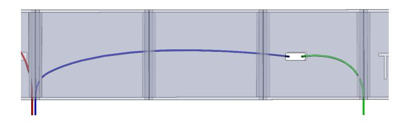
21. Feed the bolt plates through these holes in the driver side of the vehicle frame.
