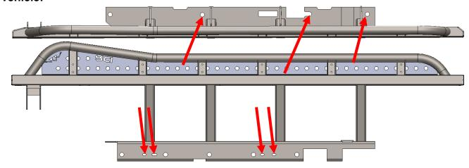
5. With the holes aligned, install four (4) M8 bolts with four(4) 5/16 washers in the four mounting locations on the bottom of the slider frame plate.
