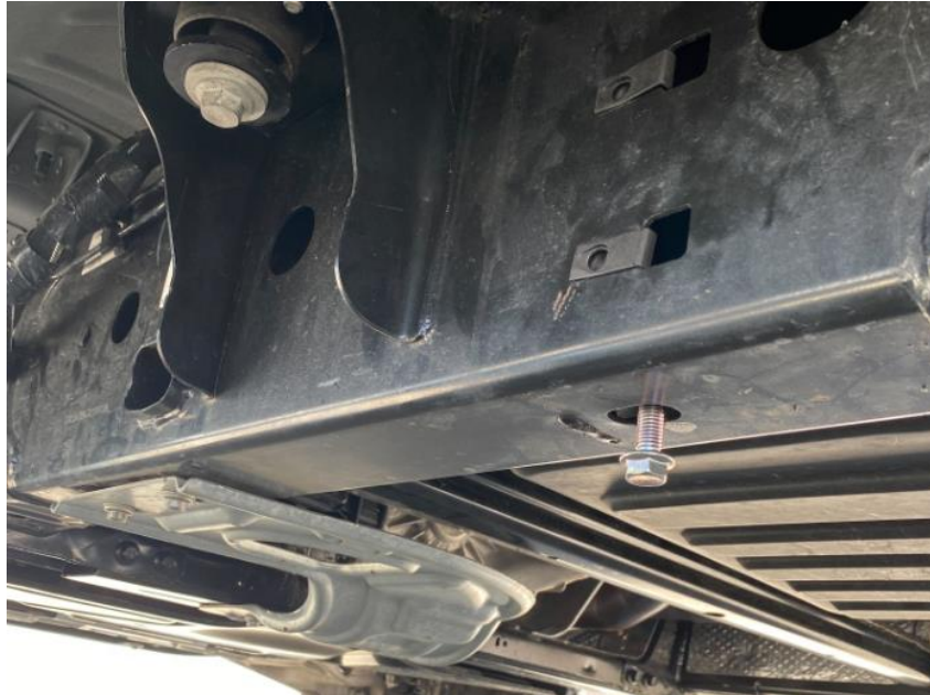
Figure 7: Preinstallation of Lower M10 Bolt
