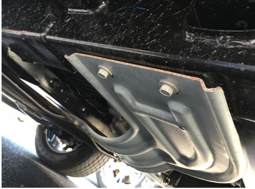
Figure 2: OEM Transfer Case Skid to be Removed.
