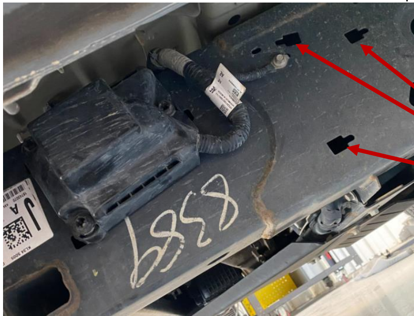
Figure 18: Slots for Threaded Stud Reinstallation
