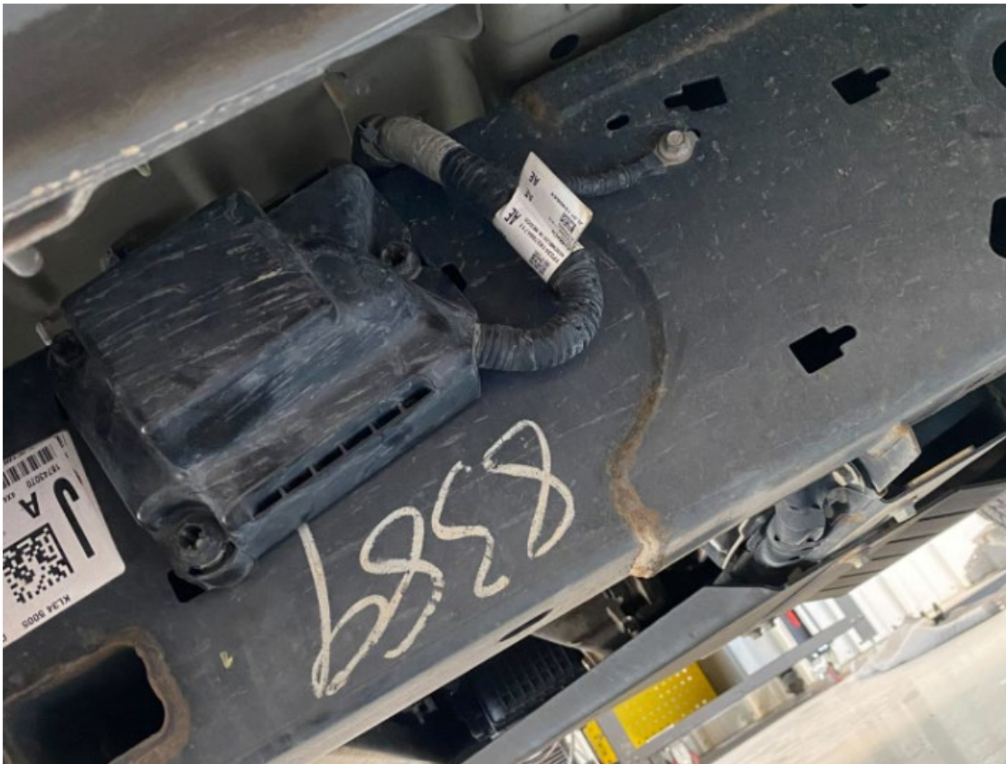
Figure 2: Fuel control box
