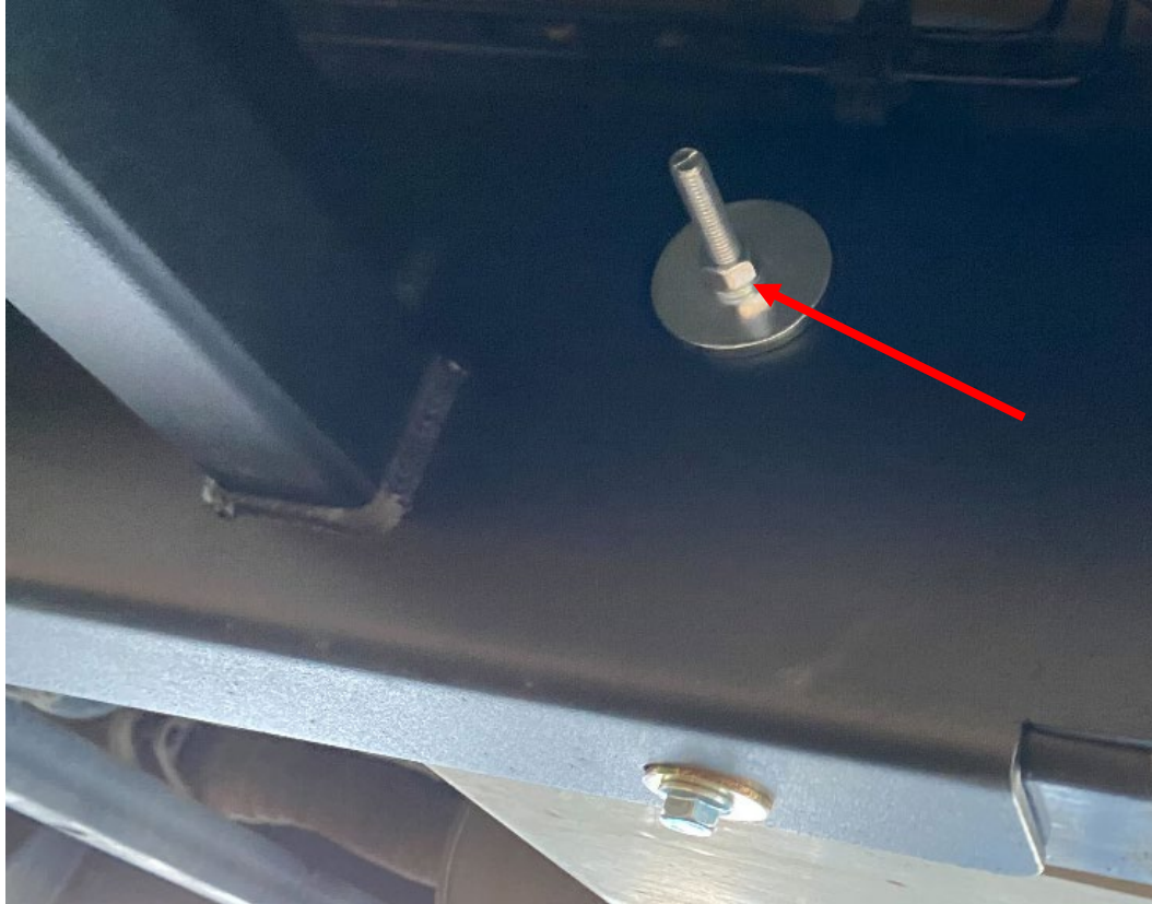
Figure 16: Correct installation of carriage bolt assembly
