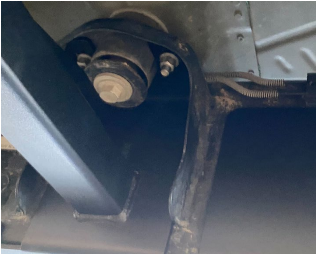
Figure 9: Body mount nuts loosely installed.
