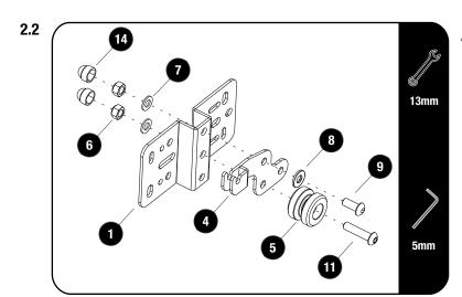
Assemble the Bobbins and Catches (Items 4 & 5) to the Awning Mount Brackets (Item 1) using a M8 x 20 Button Head Bolts, M8 x 35 Button Head Bolts, M8 x 19 x 2SS Flat Washers, M8 x 16 x 1.6SS Flat Washers and M8 Nyloc Nuts (Items 6, 7, 8, 9 & 11) as shown.
