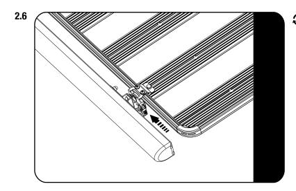
Place the loop of the latch over the hook of the Catch on the Mounting Bracket.
