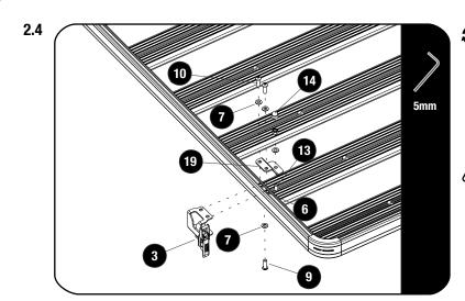
Place the Rack Mount Brackets (Item 3) over the side profile, followed be the Rack Support (Item 19) and secure using M8 x 25 Button Head Bolts, M8 x 16 Hex Bolts, M8 x 16 x 1.6SS Flat Washers and M8 Nyloc Nuts (Items 6, 7, 9, 10 & 13) as shown.
