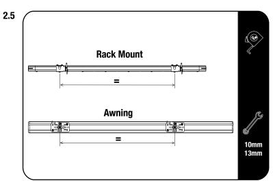
Measure the pitch of the Rack Mount Brackets. Transfer the measurement over to the Awning Brackets.
