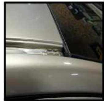
The trim is held in the front by the tab shown above and pulls up
