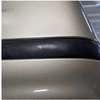
Locate the weather stripping on the top of the roof and remove
