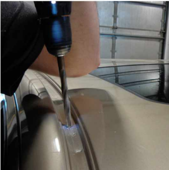
Drill one hole on both sides of the truck. The recommended hole size from plus nut is .386"-.391". The roof is approx. 1/4" thick, be very careful not to drill excessively deep as the airbags are located below
