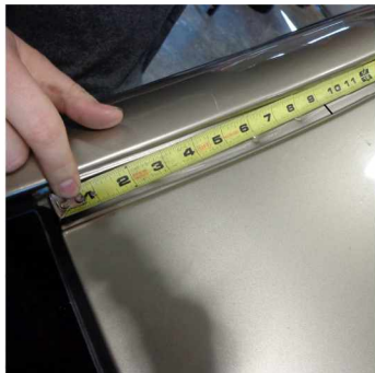
Mark off at 9-1/8" inches on the driver and passenger sides. These will act as your guide holes later in the process
