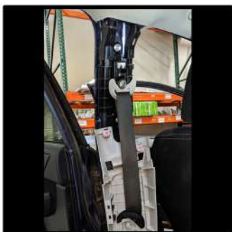
B pillar trim removed, it's held in by plastic push tabs
