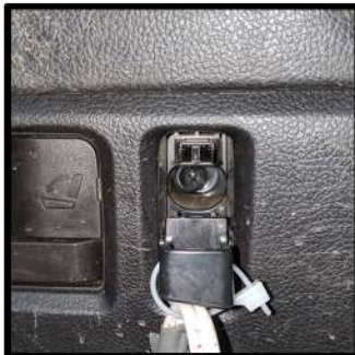
Now move to the passenger side of the vehicle and remove the screw pictured above
