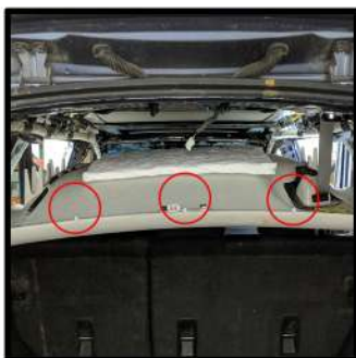
The rear is held up by three plastic push tabs, once removed The headliner will fully drop
