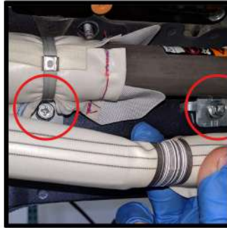
To gain better access to the nuts near the middle of the car partial loosen the screws holding the cylinder shown above ...
