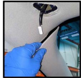
Undo plug for the in visor lights and pull out on the top of the A pillar trim
