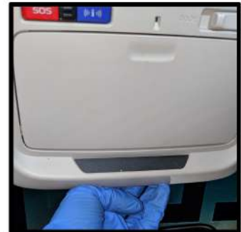
To remove the dome light console pull down and out from the front
