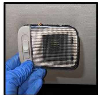
Remove rear dome light with a plastics removal tool
