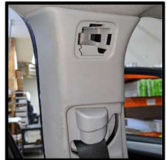
From the top and sides pull out on the B pillar plastic
