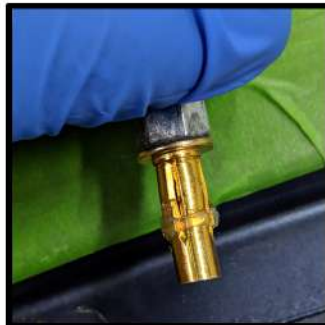
Be sure to clean any shavings away that fell thru while drilling Then apply a thin layer of silicon before inserting the plusnuts
