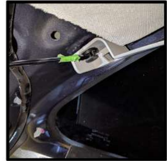
Next begin removing the trim panel surrounding the rear window by first pulling down the center of the black push tab
