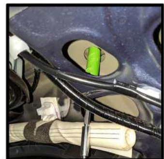
To remove the far rear roof rail nut use the access holes to reach the nut
